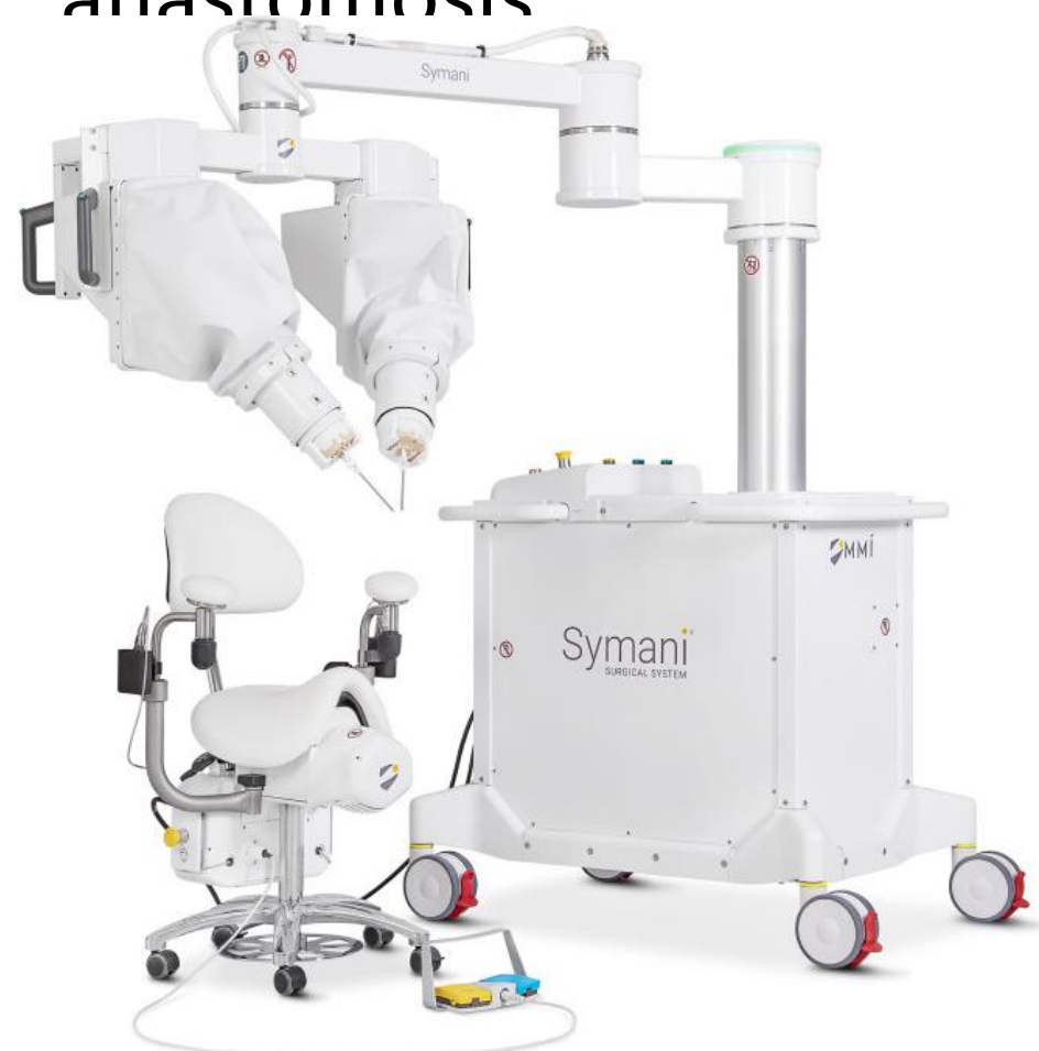
Figure 1. The Symani® Surgical System is a flexible platform consisting of two robotic arms that can be easily positioned to facilitate surgical procedures across any anatomical region.
